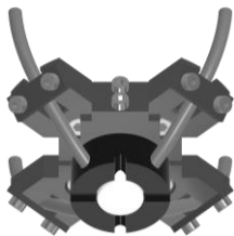
Figure 2. Sample between foils (white) in sample mount and optical fibers
